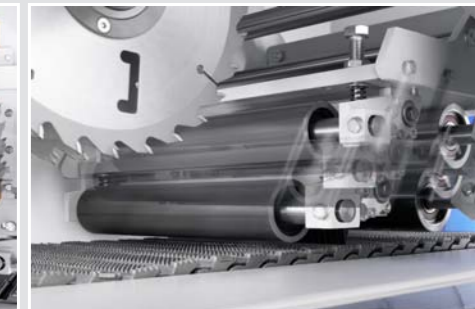
Motorized height adjustment of the pressure unit: great operating convenience
