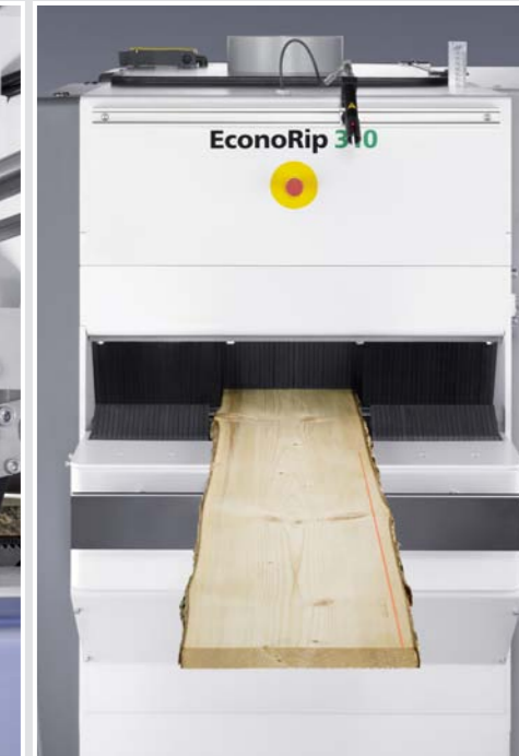
Laser for indicating cuts: see what is being sawn
