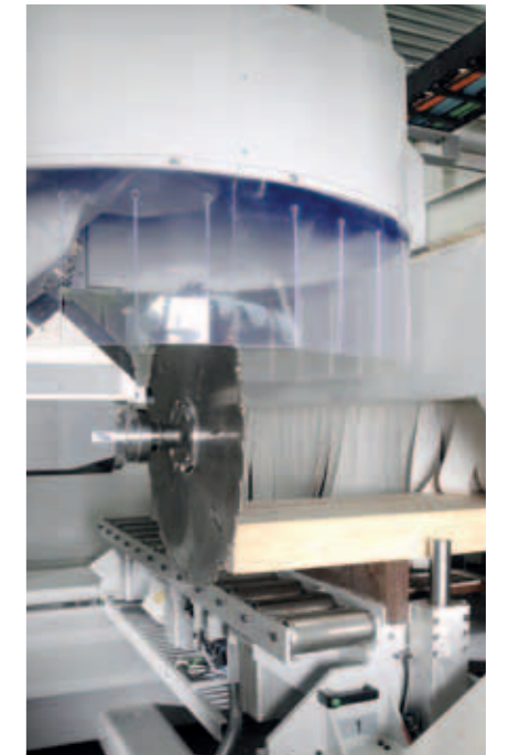
Glulam-machining (up to 50 m) with a 5-axes working unit (spindle 55 kW, saw blade 800 mm).
