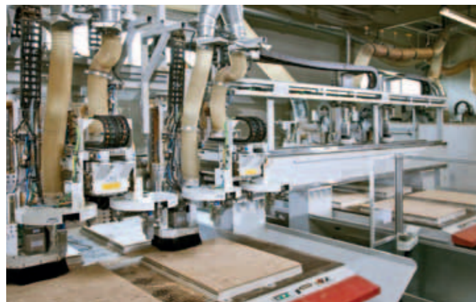
ECO with 2 tables and 4 units for nesting, including tool changers with 12 places to move along.
