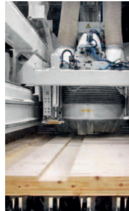
VISION-III-T for machining walls for wooden houses up to dimensions of 13,500 x 3,200 x 250 mm.
