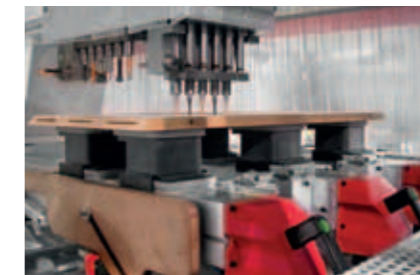
Machining of a furniture body part with a 15-spindle drilling unit in an ARTIS.
