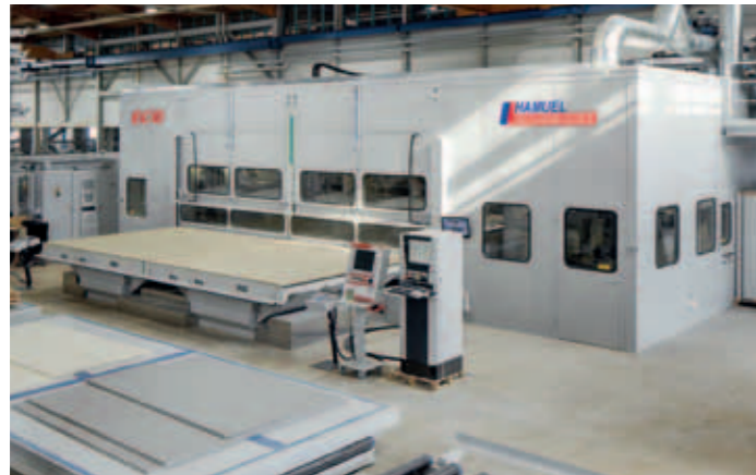
Machining centre type ECO with tables that can be coupled for the processing of plate sizes up to 3.3 x 7.0 m.
