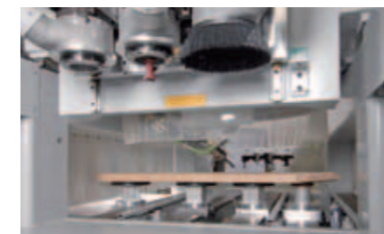
3x positionable milling motors mounted at the front of the Y-slide and connected to the cardanic working head.
