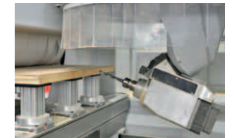
Cardanic 5-axes working unit (spindle 24 kW, undercut -20°) for the machining of solid wood.
