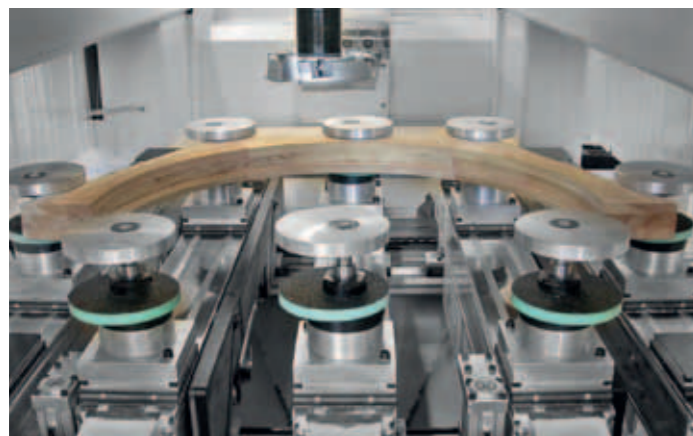
Automatic beam table with individually controllable clamping devices for the machining of round window arches.
