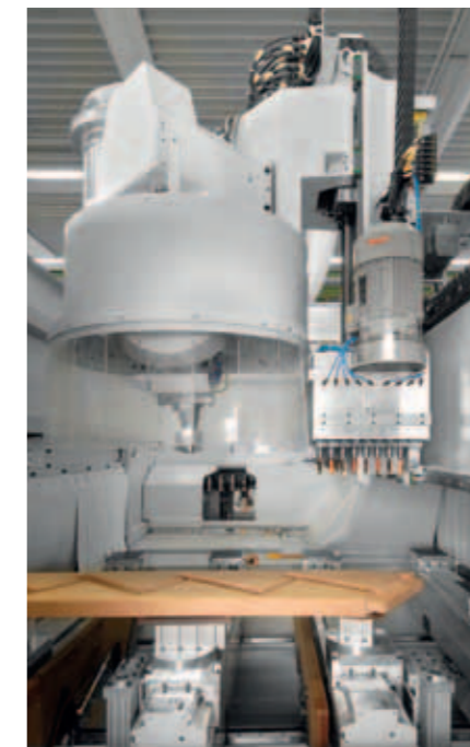
ARTIS-X with automatic beam table, multi-spindle drilling unit with 25 places and chain tool magazine with 36 places.
