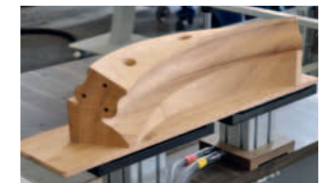
Interpolating 5-axes machining. The handrail is completely machined and cut to length. Design and programme established by your software company.
