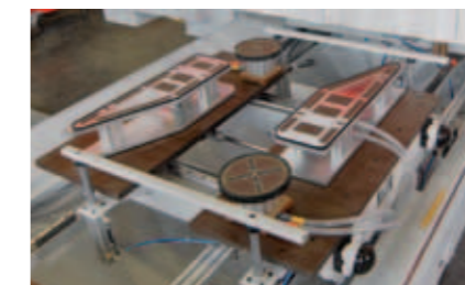
Clamping device left and right for the alternate machining of steps. Suction cup design: central suction cup and thus no need to change the device.
