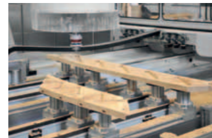
Machining of staircase strings on an ECO with 2 automatic beam tables.
