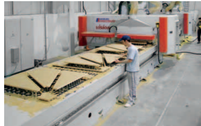
VISION with pin table: 12 corner steps are machined within 12 minutes (including set-up).
