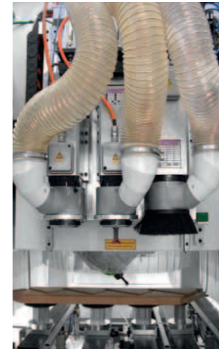
Working units of a VISION-ST (staircase production) with 5 axes and three additional milling motors.
