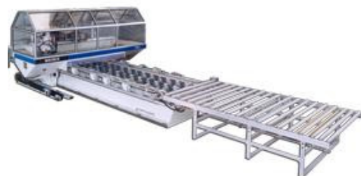
Pic. 5 High-productivity work cell with automated loading and unloading on roller tables, for the production of thermo-insulating panels
