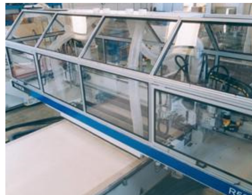
Pic. 3 Safety enclosure all-around the head unit
