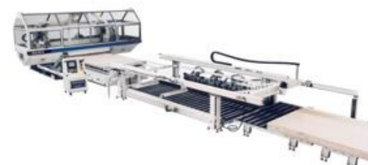
Pic. 4 High-productivity work cell with automated preloading, loading and unloading, for the production of upholstery frames
