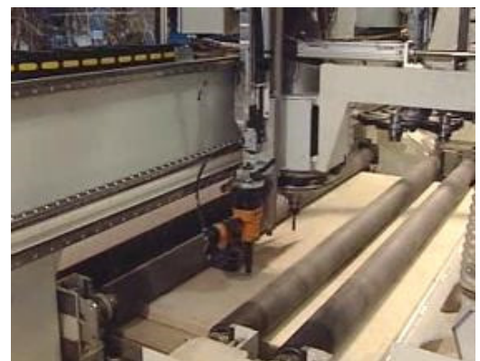
Pic. 2 Pressure rollers with dynamic intervention
