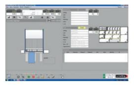
Display of the current cutting pattern, the cut, the order, and the material on the operators screen.
