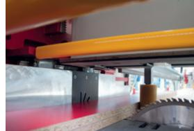
Both the saw unit and the feed trolley are equipped with the special Schelling high-performance round rod guides. This ensures precision and reduces maintenance costs.
