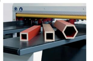
Because boards are cut to size and mitre cuts are performed simultaneously on only one machine, there is no need for handling from one saw to the next.
