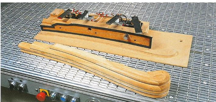
Inverted "T"-shaped grooves and a series of threaded holes provide perfect fixing for all holding-down devices.
