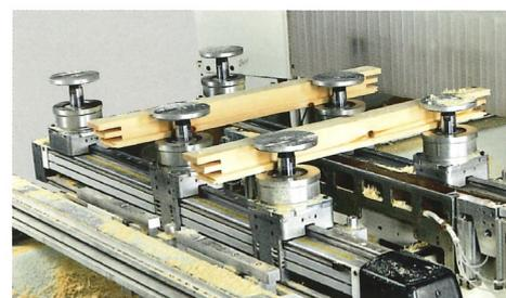
Quick release rotating clamps and double movement lifting units make it easy for assembled sash positioning and for trimming operations.
