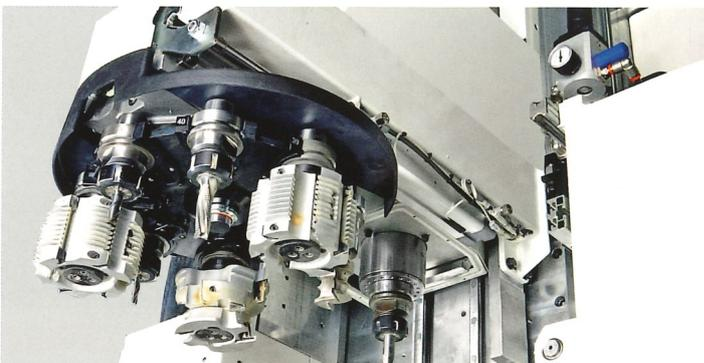
**PBTC:** Auxiliary routing unit with automatic tool changer to ensure the production cycle and chip to chip times are faster.
