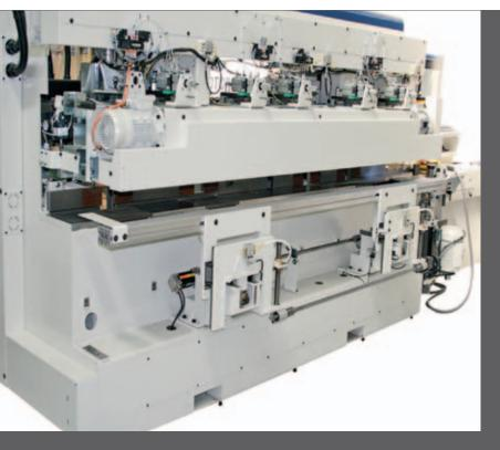
When pieces with a marked left profile or of considerable thickness need to be machined, the left guide can be equipped with horizontal and vertical electronic positioning in order to ensure machining precision and optimal finish.
