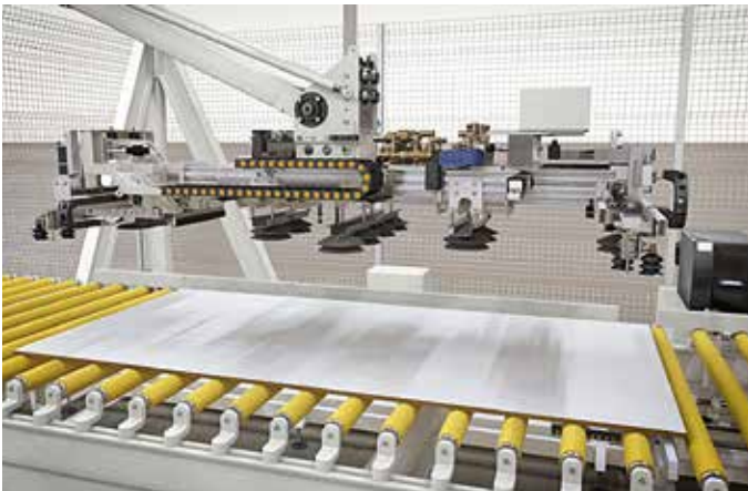
The suction cup arm, capable of rotation, automatically adapts to the different lengths and widths of the panels to be picked up, it can be equipped with the device to adjust the panel positioning. In the presence of a beam saw, panels can also be loaded transversally.
