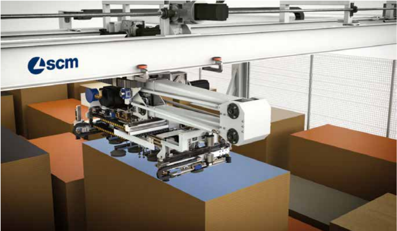
Suction cup arm designed to include thin panel management devices.
