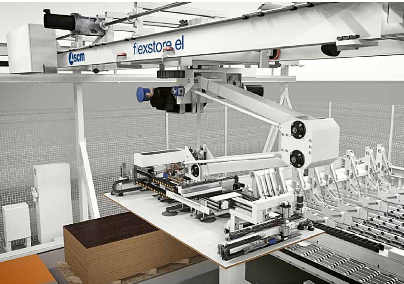
Secure, precise panel transfer. The suction cup arm has a device for pneumatically-operated panel front detachment, and a weight detection device for checking that separation has been achieved. Cycle and thin panel management devices.
