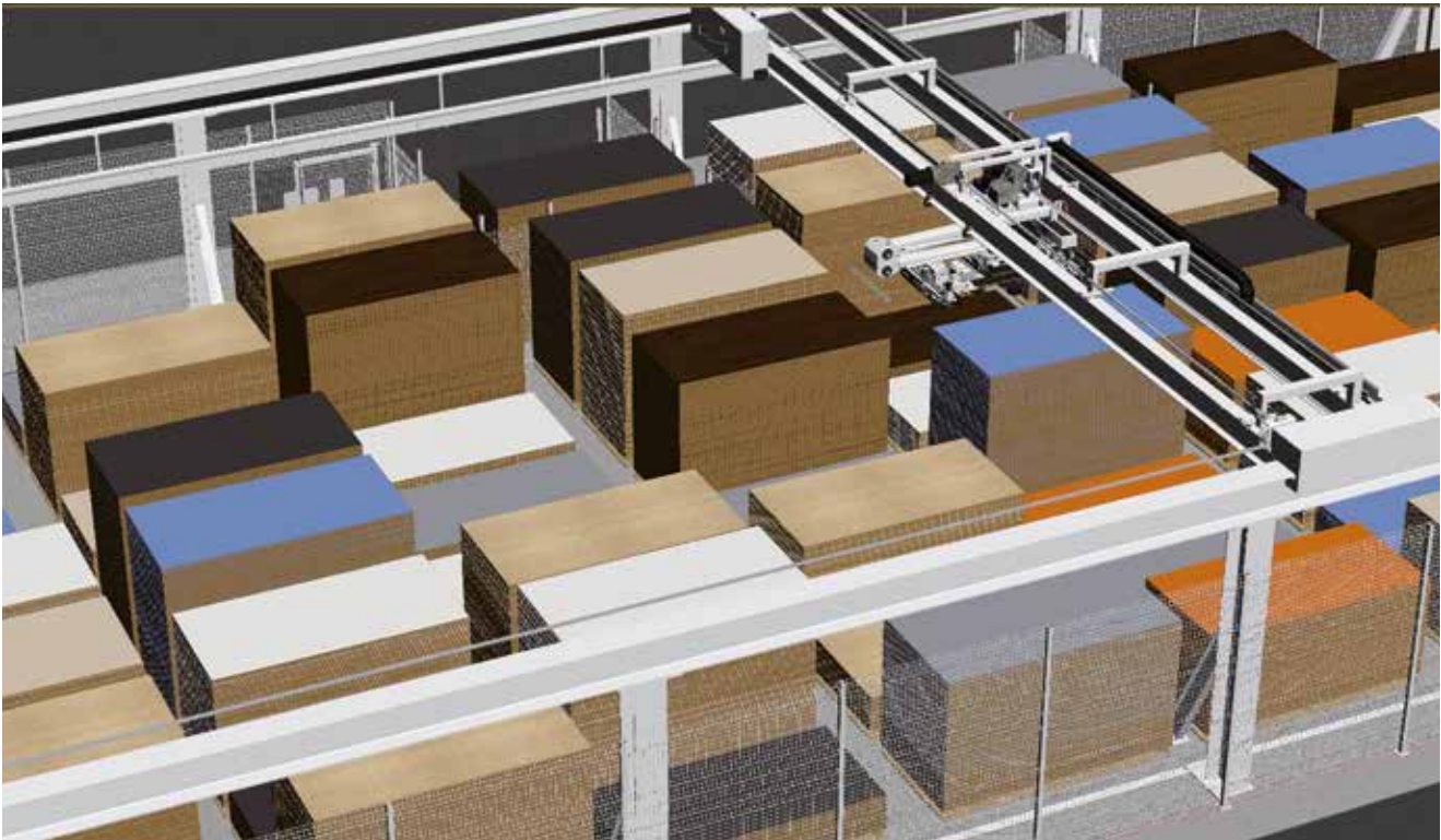
The steel structure allows vibration-free movements even in large storage systems.
