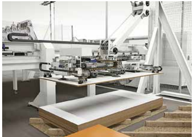
The suction cup arm, capable of rotation, automatically adapts to the different lengths and widths of the panels to be picked up, it can be equipped with the device to adjust the panel positioning. In the presence of a beam saw, panels can also be loaded transversally.
