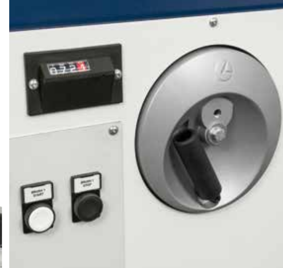
Simple working Machining units lifting by means of handwheels and numerical readout.
