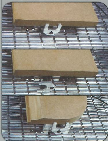
Reference stops automatically recover the portion of stock removed.
