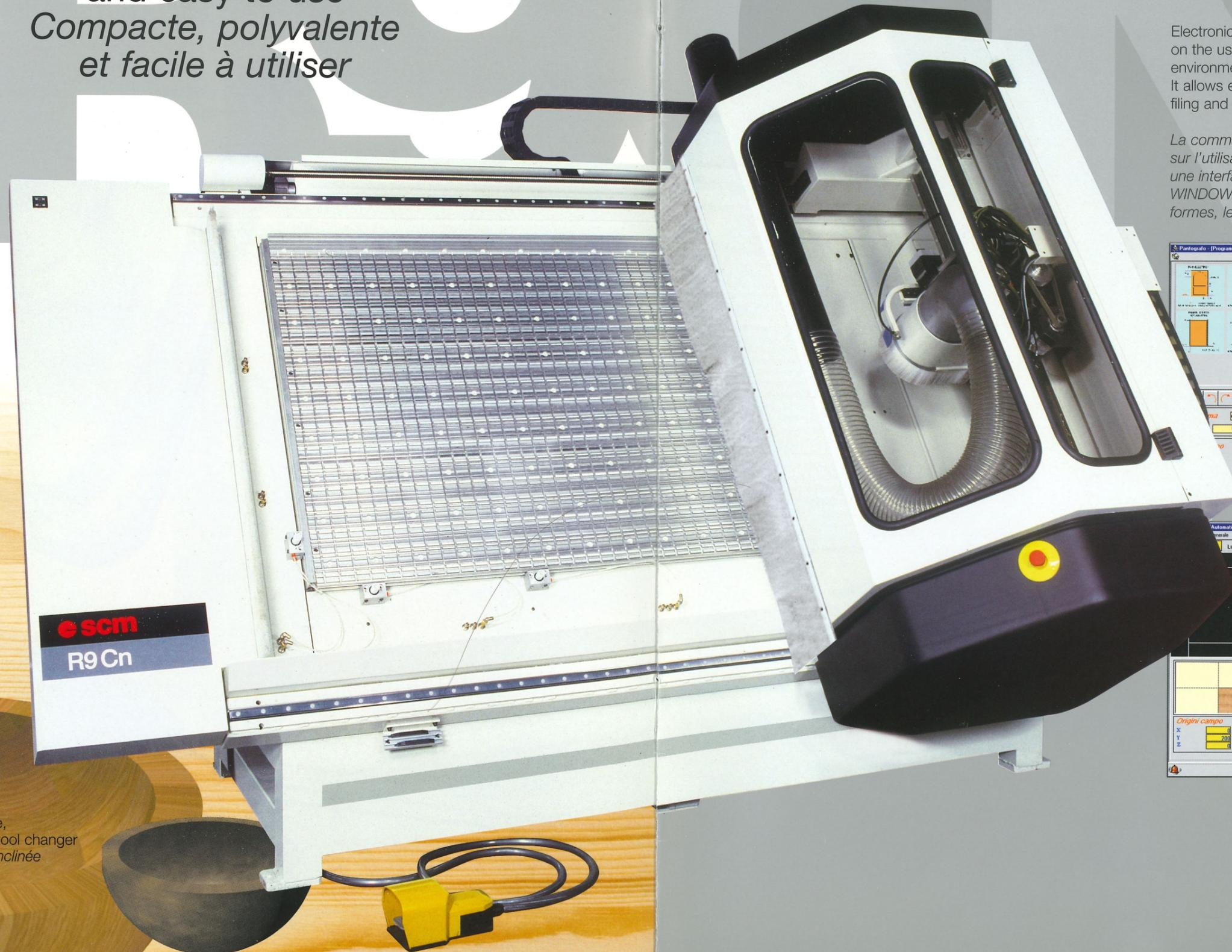
Electronic axis management is based on the use of an industrial PC with WINDOWS environment operator interface. It allows easy shape configuration, filing and subsequent use.
