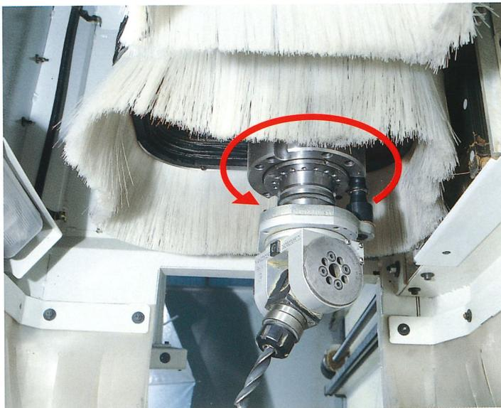
**Vector rotary axis** for routings, sawblade cuttings and drillings on tilted axes using angle drive heads
