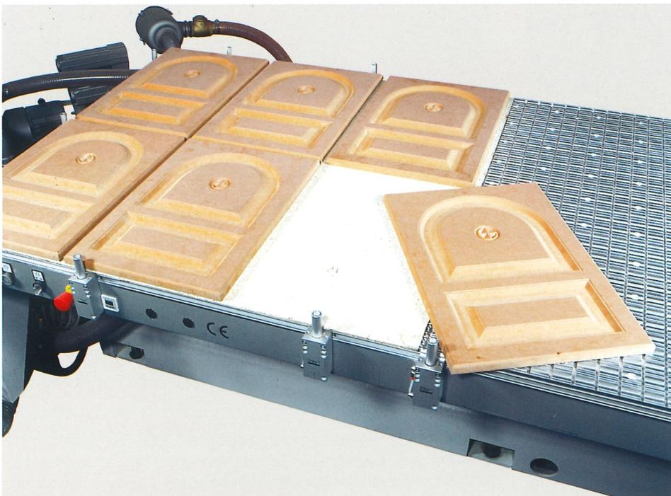
Ideal for aspiration clamping because it ensures high vacuum capacity, constant in each worktable area-
