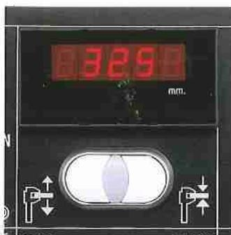
Motorized positioning for worktable belt with digital readout of working thickness (standard).
