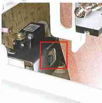
Electronic control for feed belt, with a photocell equipped with a presence detection system (standard).
