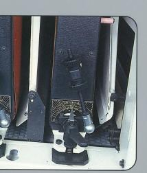
Sanding units with individual adjustment "Quicker, easier set up".
