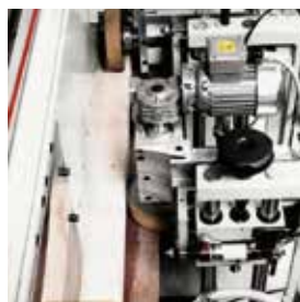
Station for glue application on flat surface
