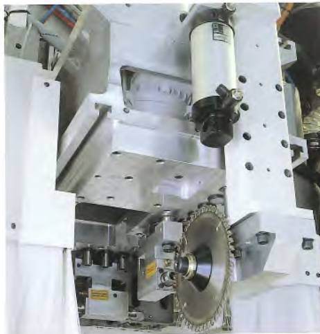
Drilling unit with 12 and 15 vertical and 6 horizontal spindles which includes saw blades cutting: max. diameter 120 mm (optional).
