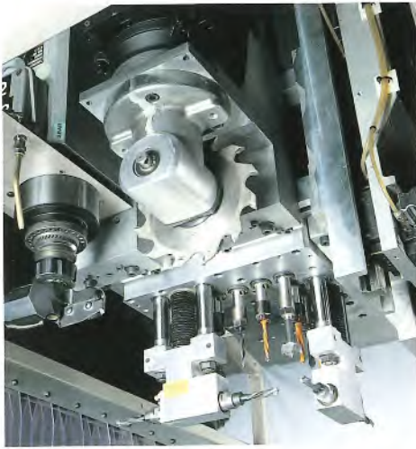
Operating unit with 10 vertical and 4 horizontal spindles (standard).
