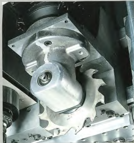
Blade unit fixed on either the X-axis or Y-axis with motor power of 2,2 kW and blade diameter up to 160 mm. Automatic NC unit for positioning on the X-axis and Y-axis with motor power of 2,2 kW and blade diameter up to 200 mm.
