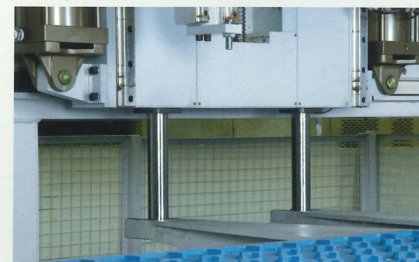
New full servo Pallet Change System using axis drive motor.
