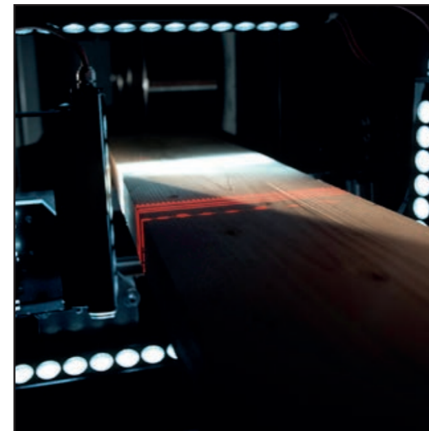
► The multi sensor scanning technology scan the workpieces for best wood utilization.
