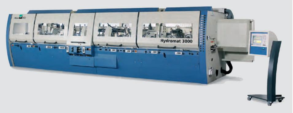
Hydromat 3000 is the planer/moulder for you who wants to produce mouldings and cladding at a higher speed and with the best possible quality. You can produce up to 20.000 m³ per year and shift, depending on batch size and wood dimensions. Optimal surface quality is obtained thanks to the solid cast-iron stand that ensures a vibration free run also at high feed speed.
