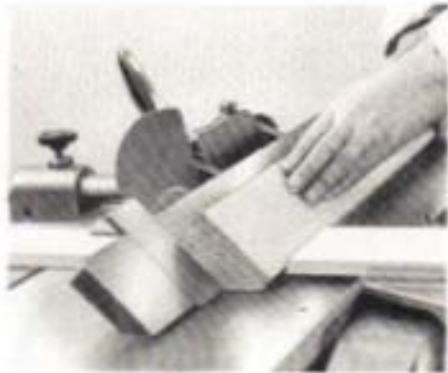
Accurate Beveling A conveniently positioned indicator shows the exact angle of the fence for accurate beveling.
