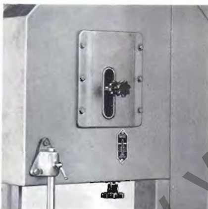
Convenient hand wheel blade tension and tracking adjustments for correct saw setting. Scale indicates tension for varying widths of saws.
