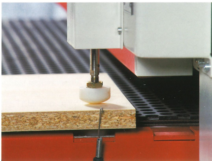
Automatic workpiece thickness measurement (AWTM) Universal lamella tensioning roller
