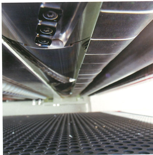
Knife planer with kickback protection
