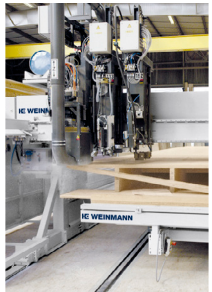
Fully automatic sawing
