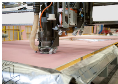
Processing gypsum plasterboard
