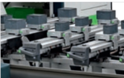
ATS (Advanced Table-Setting System) For the quick and easy manual positioning of the clamping systems.
