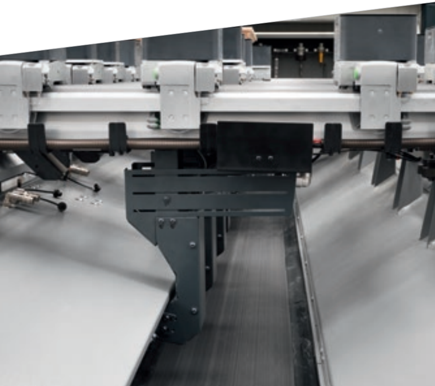
Motorised conveyor belt for the removal of chips and waste.
