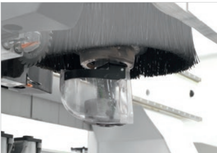
NC-controlled deflector (chip conveyor).
