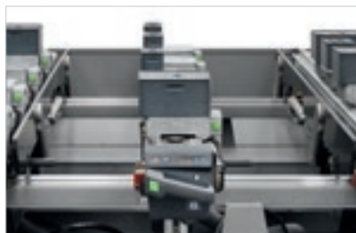
SA (Set Up Assistance) For the quick, easy and controlled manual positioning of the clamping systems. The linear sensors in the work table, along with the collision control function, reduce the risk of collisions
