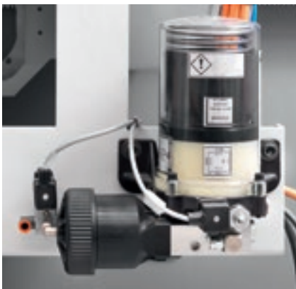
Automatic lubrication boring head BH29 2L.
