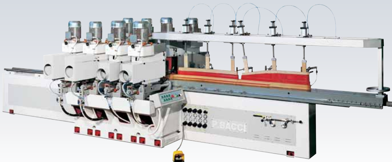
FC8 Fresa-Levigatrice a 8 teste operatrici Copying sanding shapers with 8 operating heads
