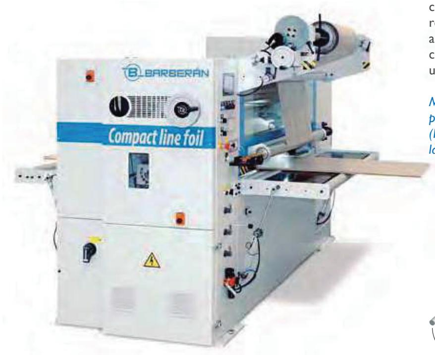
Single sided laminating machine for the application of hot melt glues on foils. The machine includes an unwinding set, a calender with cold NATURAL RUBBER rollers for the immediate application and pressing of the foil and a rotative cut system to separate the boards when using certain kind of foils.
