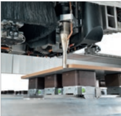
Cold or hot air blower unit to brighten up the colour of the edgelanding strip.
