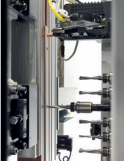
Detail of panel blocking system for boring and dowel insertion.
