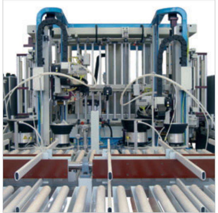
Detail – Side view of the machine with boring and glue & dowel inserting units.
