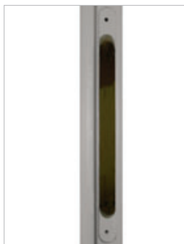
Boring and routing processing for lock slot.
