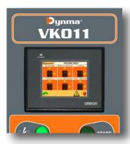
VK011Standard version equipped with a programming touch-screen. to monitoring and selecting all functional parameters, pressing forces, type of maneuvers, alarms and others.
