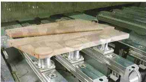
Clamping fixture for steps Fixture for all-round processing of two steps. After the separating cut, the two steps are moved apart. Different circular suction cups are available as clamping elements with a clamping height of 150 mm.
