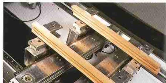
Clamping fixture for steps Fixture for all-round processing of two steps. After the separating cut, the two steps are moved apart. Different circular suction cups are available as clamping elements with a clamping height of 150 mm.
