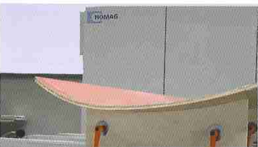
Special suction cups For clamping arched small components for 5-axis processing.
