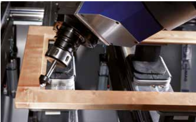
Angular cutting of a glass rabbet corner
