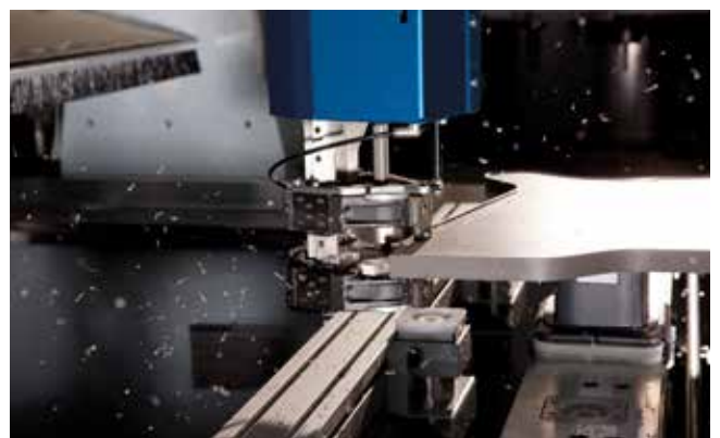
Perfect edge finish through traced combination flush routing/scraping unit
