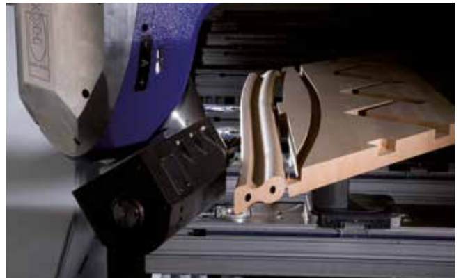
Holes for piling at a tight angle
