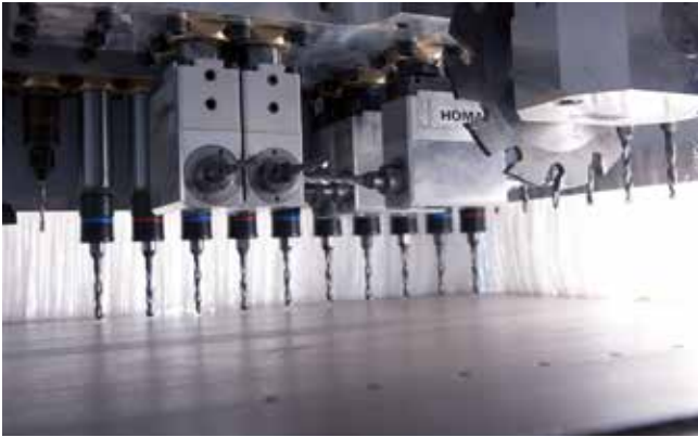
High-speed drilling technology with groove saw
