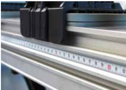
Measuring tape for positioning the suction units.
