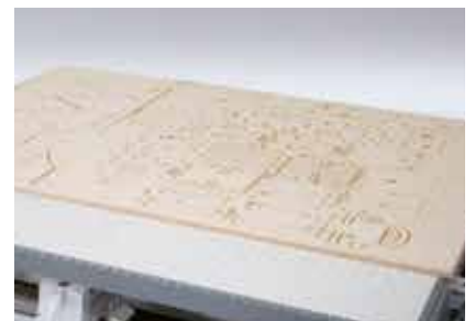
Matrix adapter plate also offers secure fixing for filigree workpieces. Shaped parts in the nesting process can also be "tailored" on a console table in an optimized way with the matrix adapter plate.
