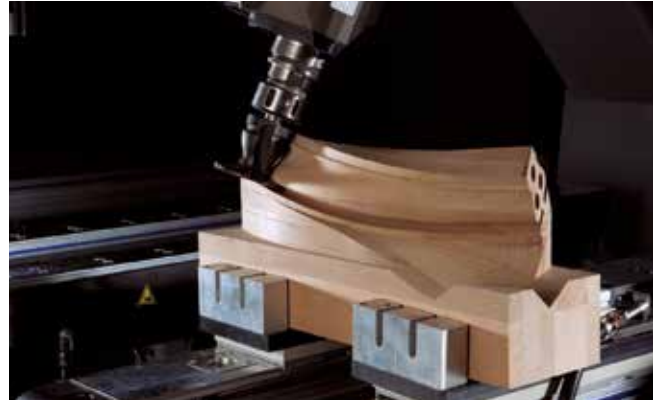
Routing a staircase handrail
