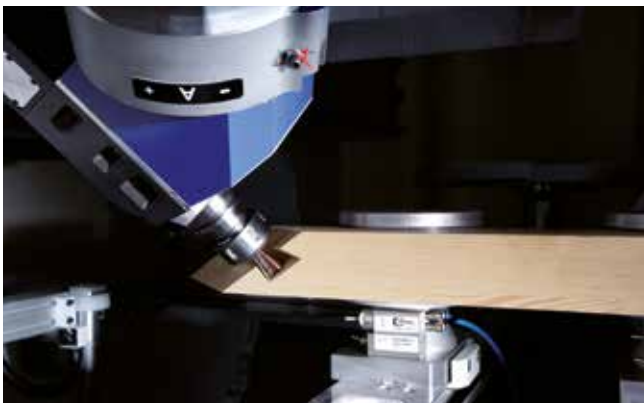
Routing a burr connection for jamb/rail designs
