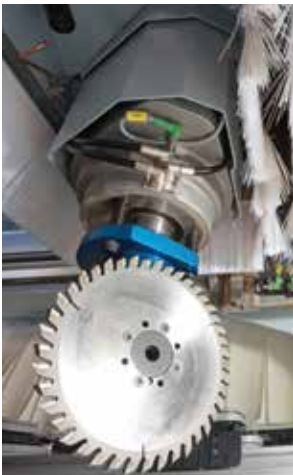
C-axis (0-360°) for the use of units
