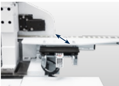
Automatic infeed fence adjustment Program-controlled precision adjustment with precise infeed fence adjustment by means of servo axis. With EDGETEQ S-380, S-390, S-500. Photo = EDGETEQ S-500.
