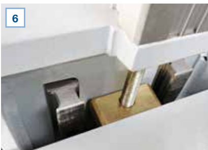
6 Linear guide for precise adjustment of the top spindles for optimal work piece quality
