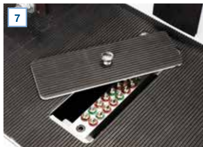
7 Accessible central lubrication at machine front
