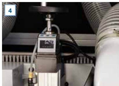
Review of radial position of tools via electronic display including target value
