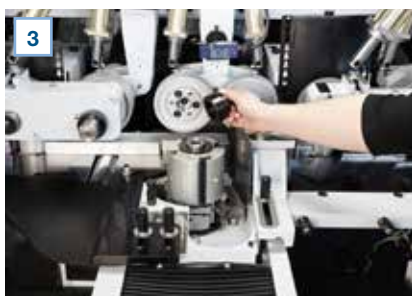
Quick and easy tool change with proven proLock tool clamping system
