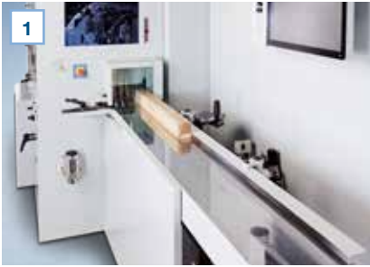
1 Harden chromed feeding table for long lasting service life
