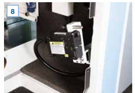
8 Automatic door lock system during process to protect machine operator
