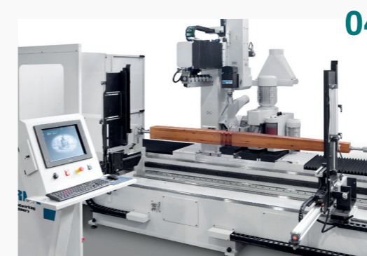
TMC-3000: A 2.5 meters wooden column been machined and sanded between centres.
