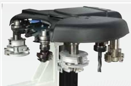
"Carousel" type tool magazine for automatic tool change. HSK F63 cone attachment.
