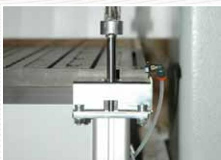
Automatic device for tool length measurement.
