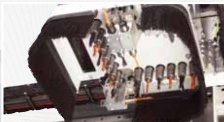
Boring head for vertical boring operations with independent mandrels.
