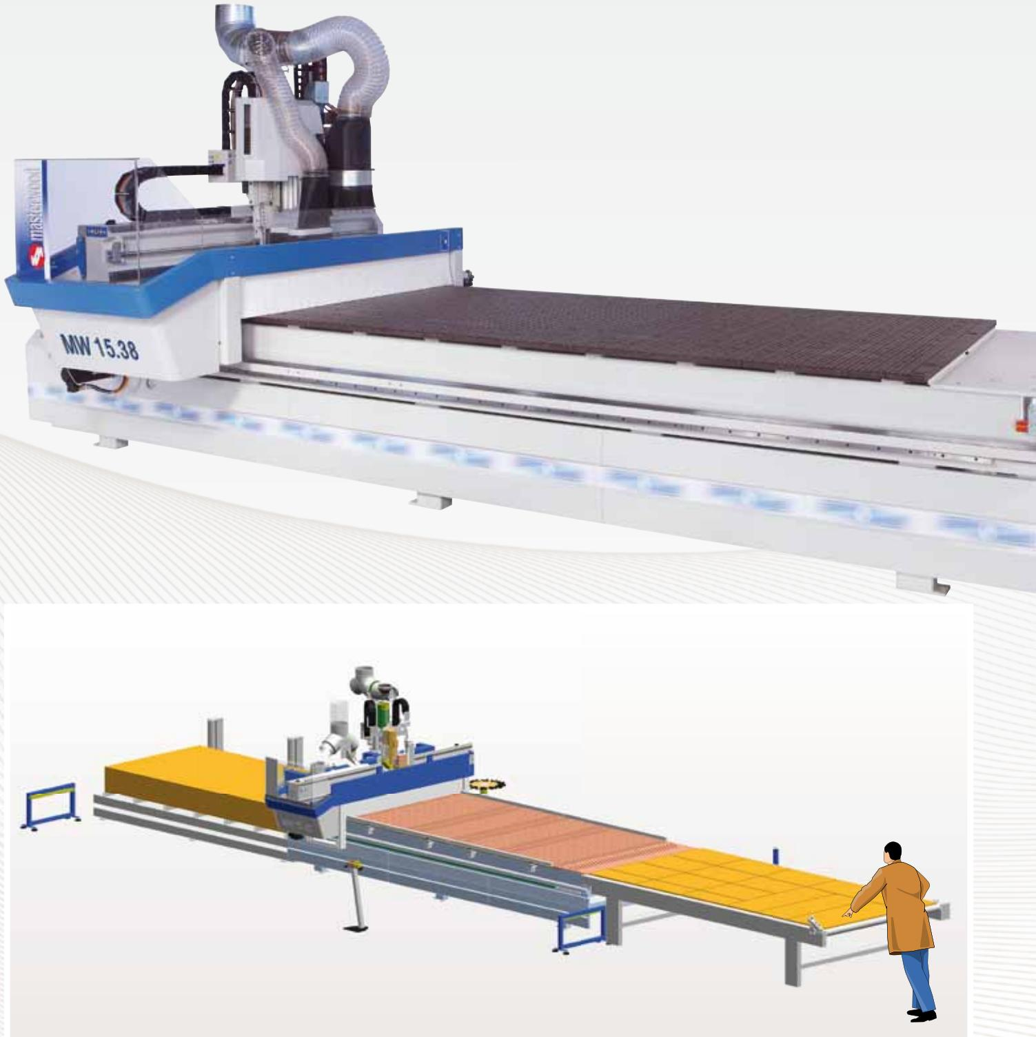
Panels loading unit with hydraulic scissors lifting platform. Automatic lifting of the platform and automatic alignment of the panel to be machined to the working table of the machine.
