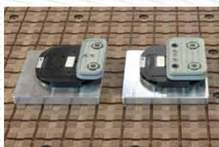
Piece locking also with vacuum cups to be positioned according to the machining requirement.
