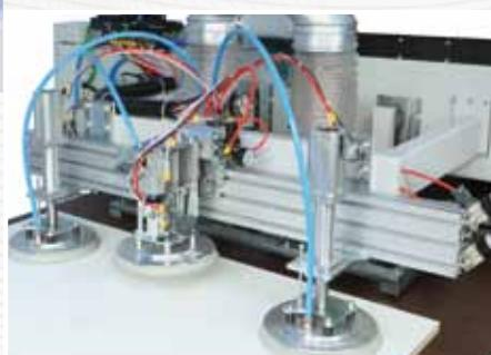
Vacuum pick up and panels pusher system to pick up the panel from the lifting platform and align it against the reference guide.
