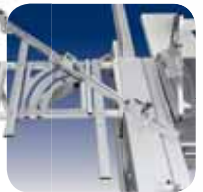
Complex to quickly carry out angular cutting with automatic self-adjustment of the stop position
