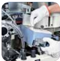
Interchangeable glue pot also for PU gluing
