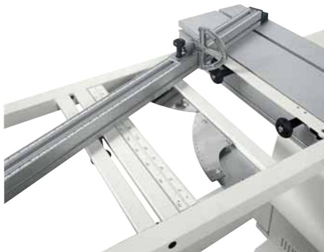
pre-set angular cutting device directly positioned on squaring frame To find rapidly the most common angles with the squaring fence. Useful for large work pieces.
