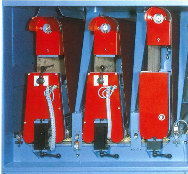
control with most powerful PLC and most modern interface for a highly efficient use of this three belt sanding machine. With automatic pressure control of sanding pads. 96 programs available!
