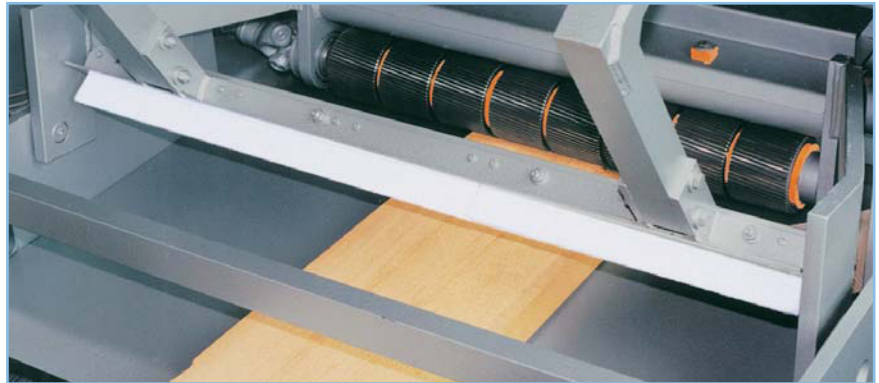
Fig. 3 Inside view of a model 18GE: Segmented top rollers, tilting sweeper
