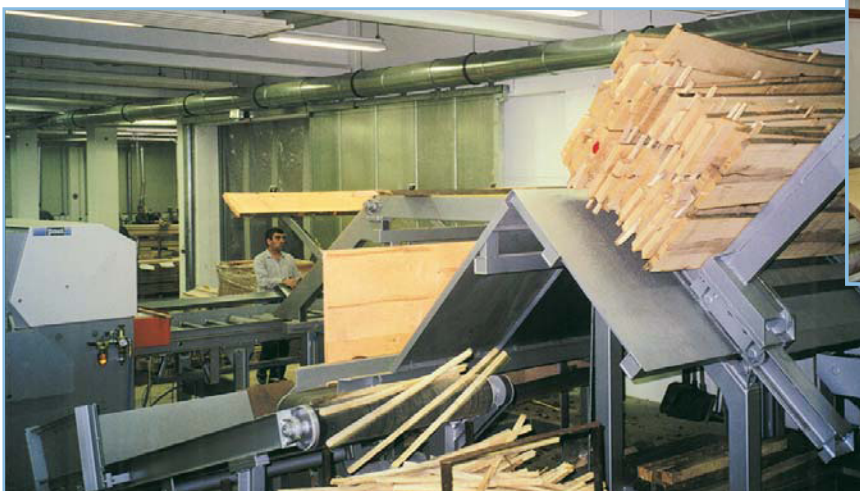
Fig. 4 Automatic destacking, stick removal and turn-over device
