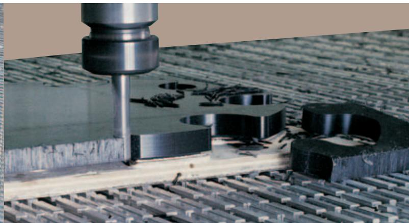
The Multi-function aluminium worktable is machined by the machine itself and guarantees long lasting, high precision and flatness thanks to its high rigidity. It is the ideal worktable for machining plastics, resins and light alloys.
