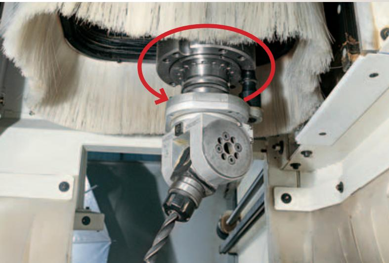
Interpolating Vector rotating axis (0-360°) enables the use of angular driven heads. The number of tool changes is extremely reduced for the best productivity and accuracy.
