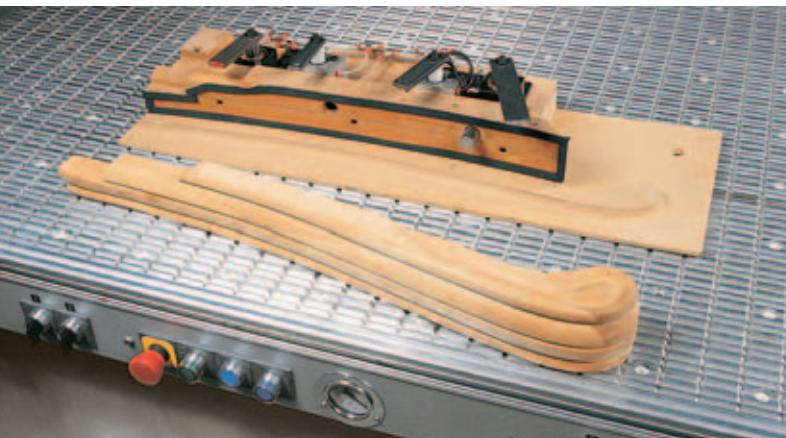
A series of threaded holes (at 120 mm pitch) provide perfect fixing for all hold-down devices.
