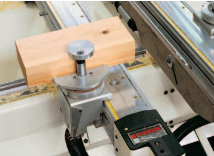
A special pneumatic clamp enables the machining of very short components.
