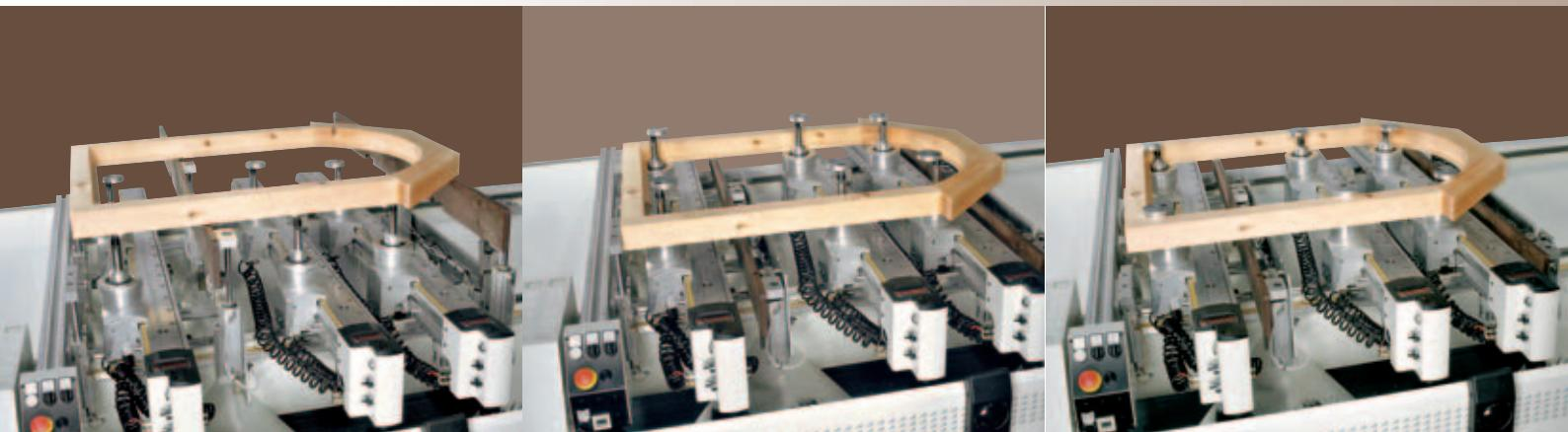
Quick release rotating clamps and double movement lifting units make it easy for assembled sash positioning and for trimming operations.
