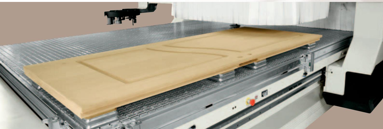
Utilising a laser positioning system, worktable set-up operations become fast and easy.
