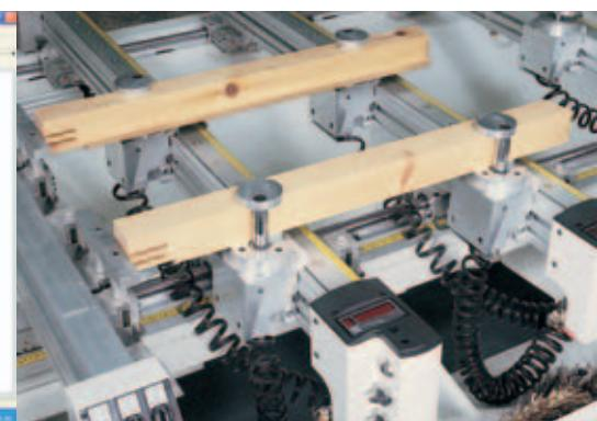
TVN SET is the ideal worktable for the automatic positioning of the bars for linear components such as doors, windows, staircases, beams, columns. Extremely simple and easy to use, it can quickly fit each window dimension. Just equip the bars with suction cups or with pneumatic clamps and then modify window dimension data in the parametric program according to size of the window to be machined. The bars automatically position themselves to fit to the new dimensions.
