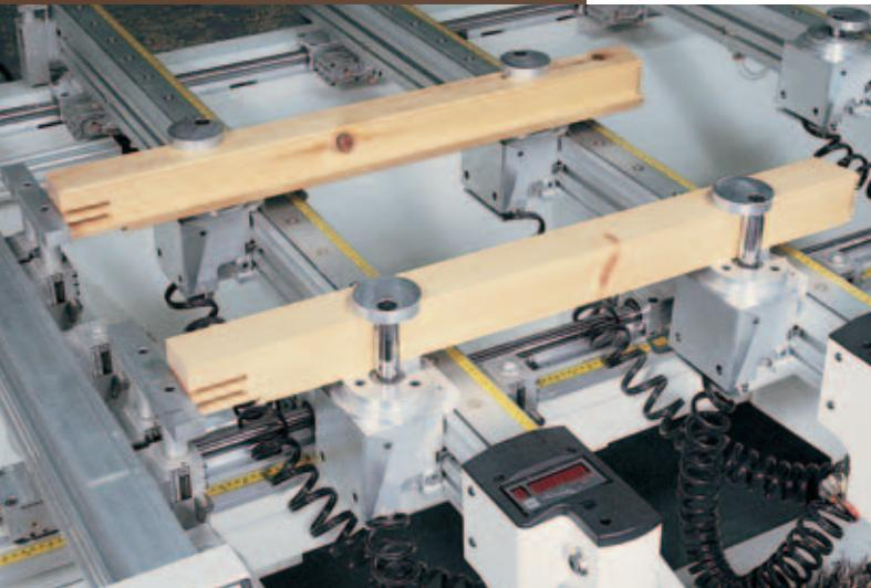
TVN worktable bars are the perfect solution for quick and safe component clamping: the bars can be fitted with quick release pneumatic clamps for maximum ease of use.
