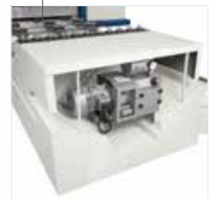
Free space on the floor with the vacuum pump integrated in the machine base.
