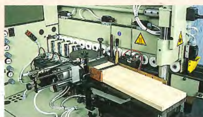
Incollaggio e pressione bordo The new gluing unit and edge pressing devices leimen + kanten aufbringen
