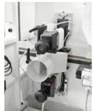
Scraping unit for the removal of the excess edge and the finishing of the profile.
