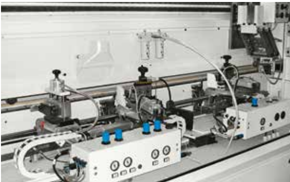
Corner finishing units for doors edgebanded on 3 or 4 sides.
