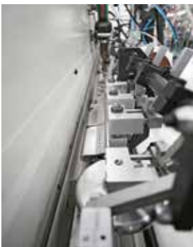
The edge pressure zone is set up as a function of the profile to be achieved with cooled shoes or a combination of shoes / rollers.
