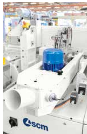
Sanding units for the finishing of doors machined with veneer edge.
