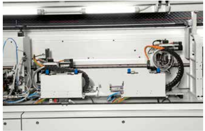
CORNER ROUNDING UNIT WITH 2 POWER ASSISTED MOTORS
