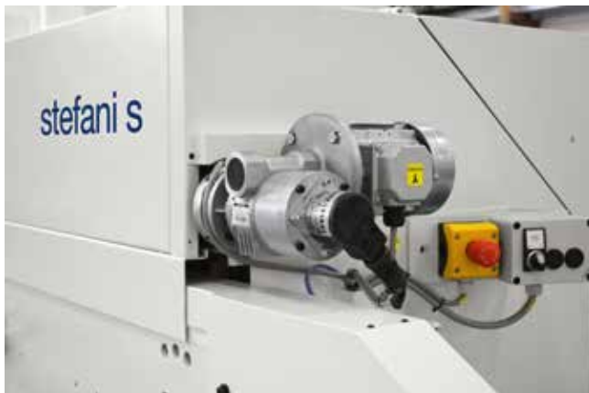
Top pressure device with NC movement (std)
