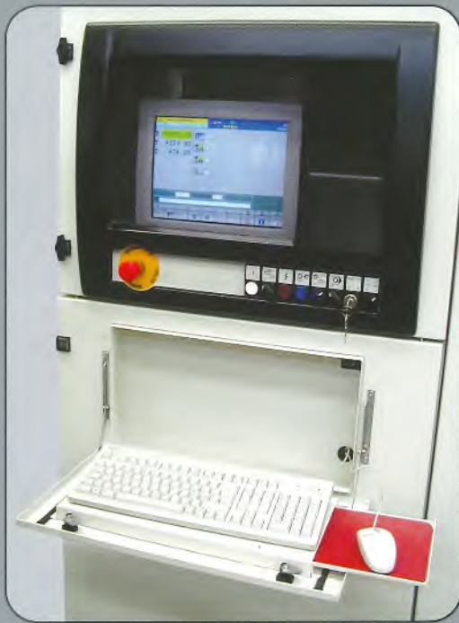
Numeric Control unit controlled from a personal computer Über Personal Computer verwaltete CNC-Steuerung
