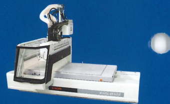
Pratix 48 NST For the nesting of components from sheet materials
