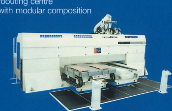
Ergon TV Fixed-gantry CNC routing centre with modular composition
