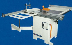
SC2 Sliding table panel saw with scorer
