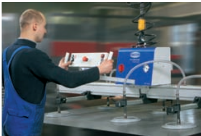
VacuMaster Comfort, 750 kg Traglast, horizontal
