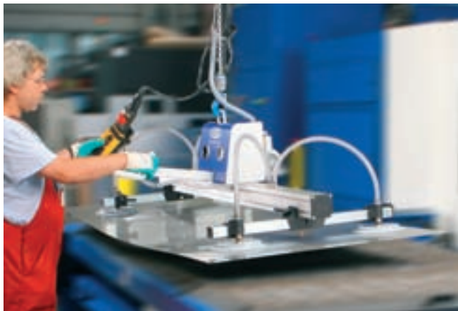
VacuMaster Basic, 250 kg Traglast, horizontal
