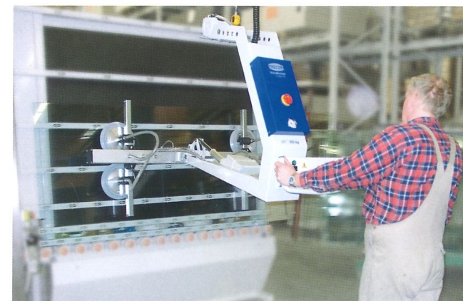
Vacuum lifting device VacuMaster Comfort being used to turn a glass sheet by 180°
