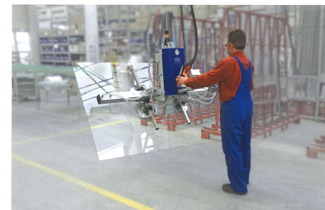
Vacuum lifting device VacuMaster Basic being used to swivel a glass sheet by 90°
