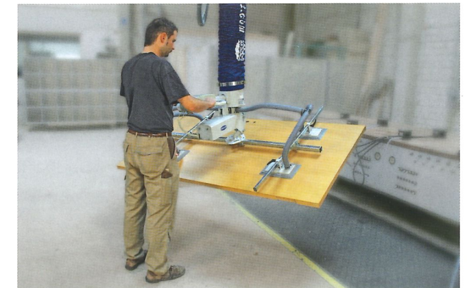
Vacuum tube lifter JumboErgo with pneumatic swiveling unit PSE for swiveling workpieces by 90°
