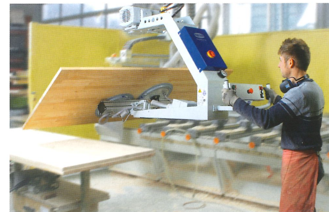
Vacuum lifting device VacuMaster Comfort being used to turn wooden boards by 180°
