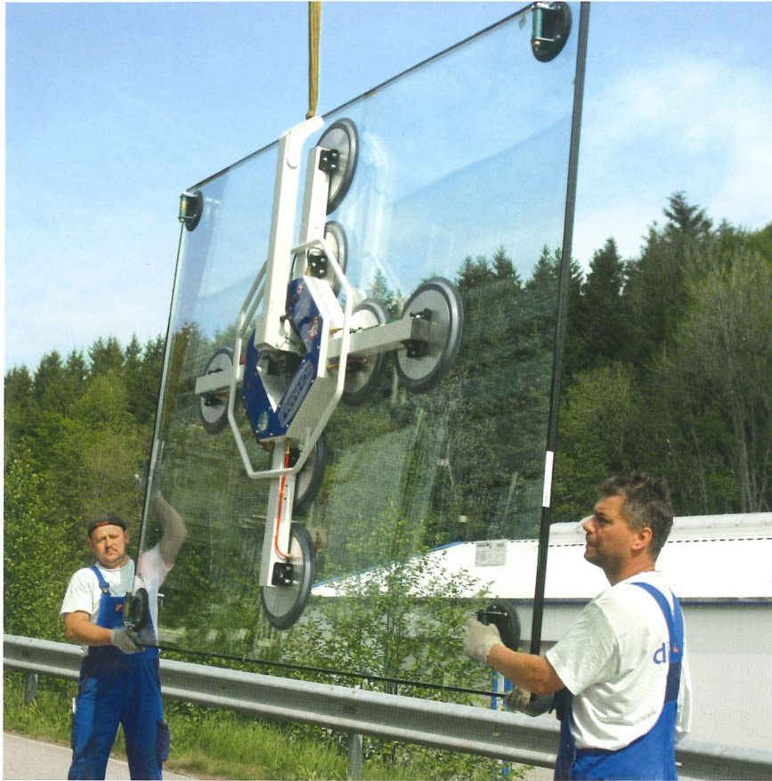
Vacuum lifting device VacuMaster Glass 600 for handling glass panes outdoors
