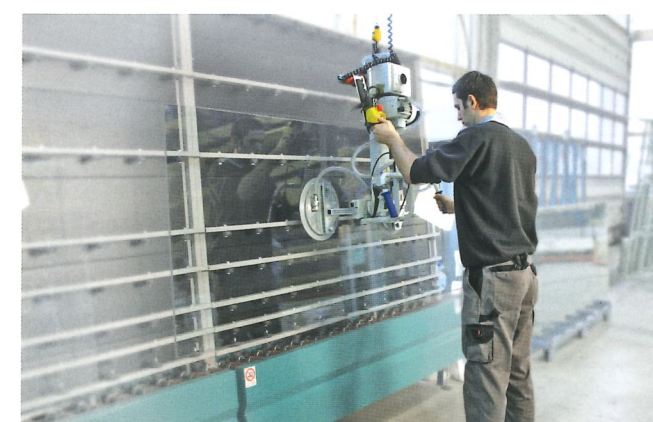
Vacuum lifting device VacuMaster Window being used to handle a glass sheet vertically
