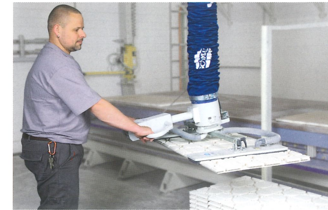
Vacuum tube lifter JumboErgo with large-area grippers FM being used to handle workpieces with gaps
