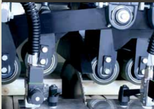
Waste and defects are efficiently removed by air nozzles and blown out at the back of the saw.
