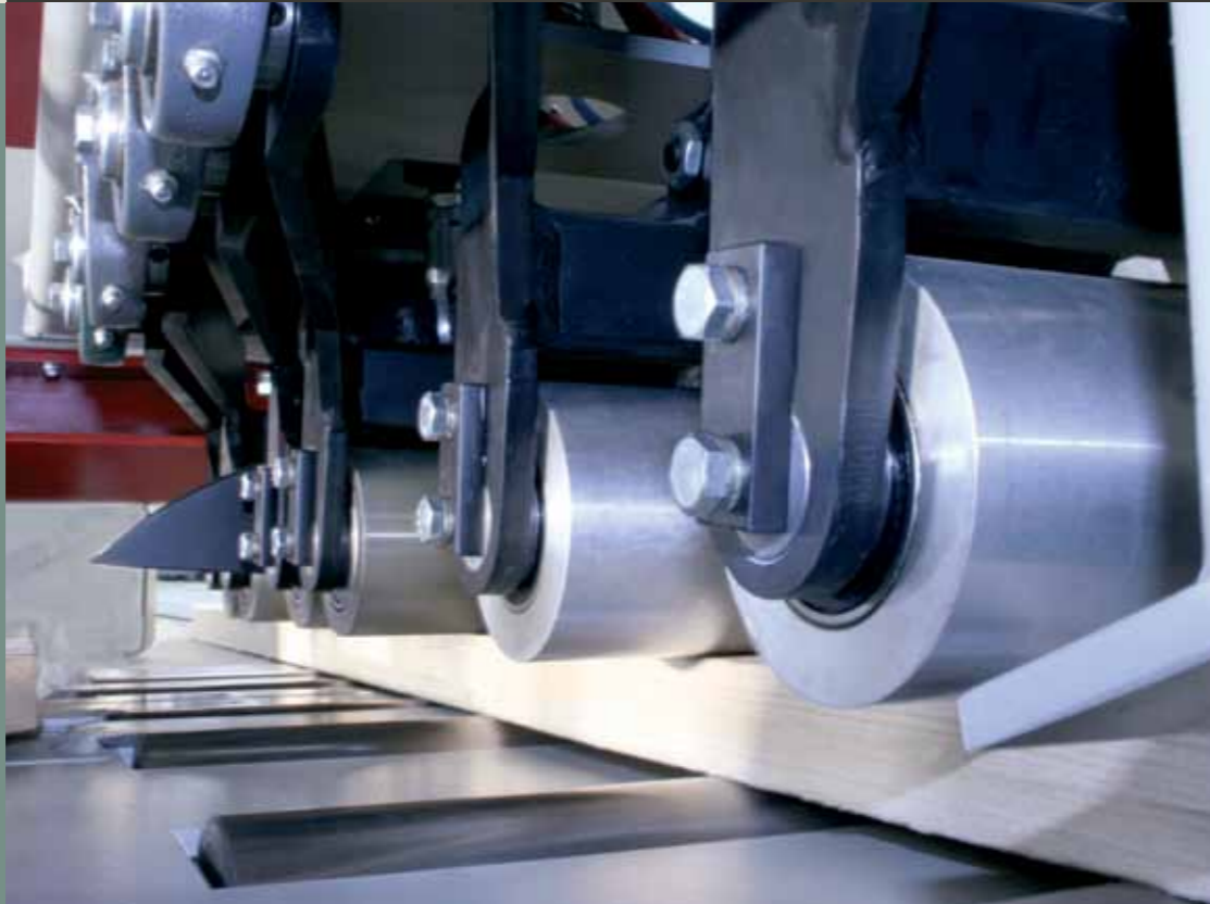
The bottom feed rollers are set high above the bed plate of the machine which allows feeding of bent or twisted timber, ensuring maximum productivity and accuracy.
