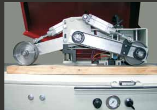
Heavy-duty measuring unit designed for a long life. The raw workpiece is measured before cutting.
