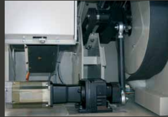
Opti-Kap 2000-3000-4000 The Opti-Kap movement is carried out by a cam and programmable servo motor which provide controllable high performance and quality cutting at all times. Opti-Kap 2000 is driven by an electrical motor. (Picture Opti-Kap 4000)
