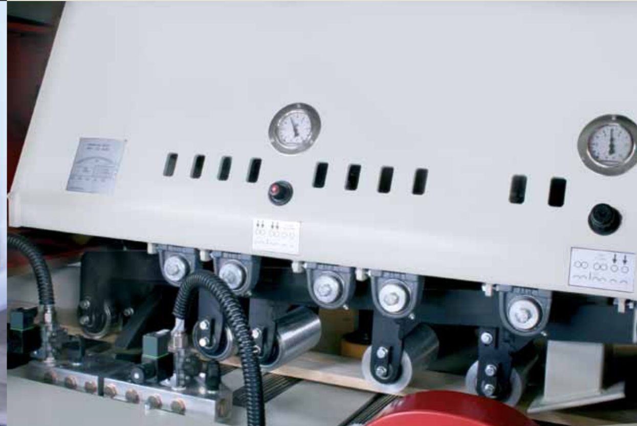
A heavy-duty top pressure construction with strong double side supported top pressure rollers. These ensure maximum contact between the workpiece and the feed roller which enables a very reliable cutting precision at high rates of acceleration and deceleration.
