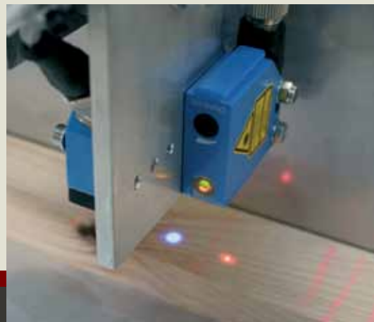
With a return speed of 290 m/min (951 ft/min) the sensors registers defects, quality and measures the board length
