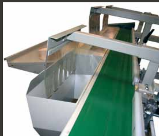
Waste chute and sorting belt
