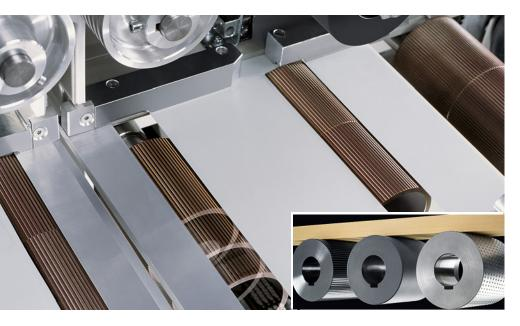
Different wood qualities impose different requirements. Thus, the feed rollers of the OptiCut 200 can be changed very quickly in order to respond to the respective requirements. Rough and planed qualities can now be readily processed in the same shift, and resincoated rollers are easily cleaned for consistently high performance in every shift.
