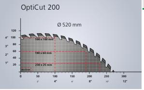
Attention! Bend and differing wood dimensions have to be taken into account when determining a possible wood cross section. The nominal values in our technical data apply here.
