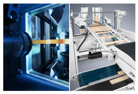
**WEINIG Scanner systems** detect fully automatically and at lightning speed relevant workpiece characteristics such as branches, cracks and structural patterns, and supply up to 4 OptiCut high-speed saws with cutting data via intelligent mechanisms while maintaining full production speed.
